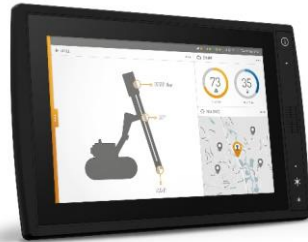
CCpilot X1400 • 14" display • Intel i5 Quad
